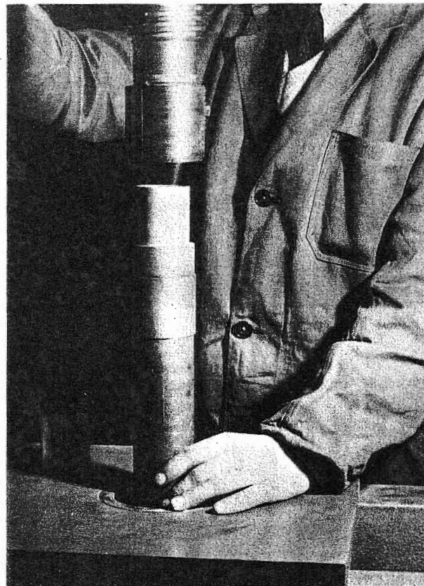
21. Warm up inner sleeve smoothly and insert new bearing insert.
