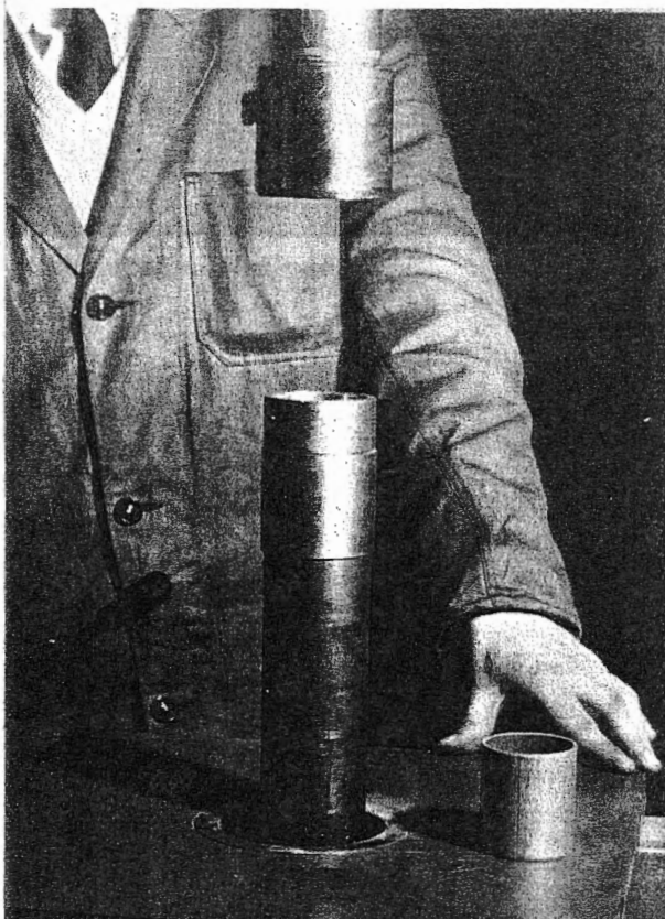
21. Warm up inner sleeve smoothly and insert new bearing insert.
