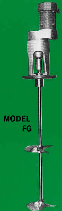
FIG. 762: Rated 150 psig @ 420 rpm. Seven rings of packing, a lantern ring for distribution of lubricant, and a packing gland for adjusting packing.
